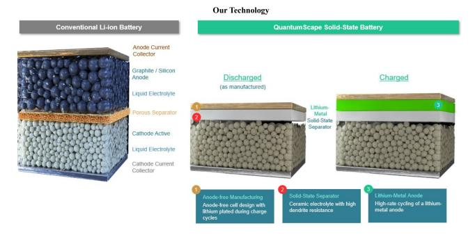
Our proprietary solid-state lithium-metal cell represents the next-generation of battery technology.
