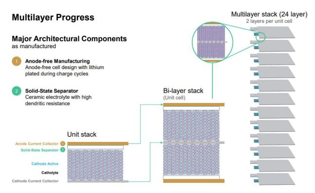
Depending upon our potential customers' requirements, our battery cell will require several dozen layers within each battery package. We have not yet built a complete multi-layer solid-state battery cell in the dimensions required for automotive applications but have announced the results of our single-layer, and multi-layer cells in commercially relevant areas, and in 2022, shipped 24-layer A0 prototype battery cells to multiple automotive OEMs for testing.
