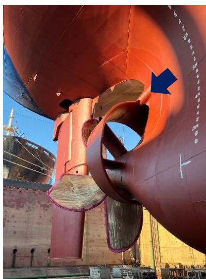
A Mewis duct was installed and a high-performance hull coating was applied on Dachshund
