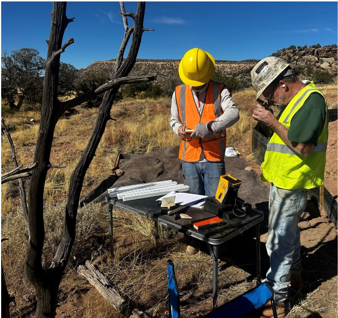
Photo 3: Thor's Geology Team logging drillhole and taking pXRF (V) and spectrometer (U) readings
