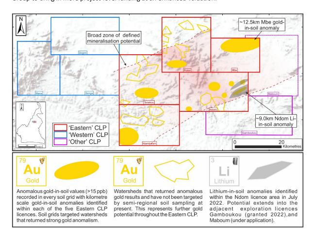
Figure 1: Simplified summary of the prospective areas across the CLP. Lithium anomalism identified to date is located in the southeastern corner of Ndom, with the Gamboukou, and Maboum licences also having been identified as having highly-prospective geology.
