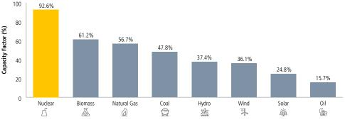
Note: Capacity factor measures the total amount of energy produced during a period of time divided by the amount of energy the plant would have produced at full capacity.
