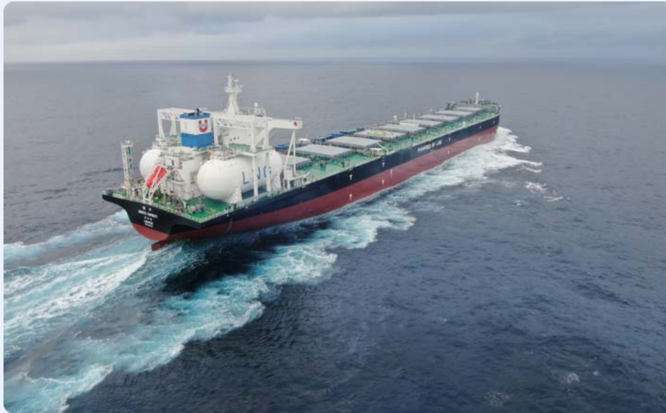
The Ubuntu Equality is the second of 10 LNG dual-fuelled Capesize+ vessels in our chartered fleet. Our LNG dual-fuelled Capesize+ vessels are estimated to deliver a 35% reduction in CO 2 emissions compared with similar vessels fuelled by conventional marine oil fuel.
